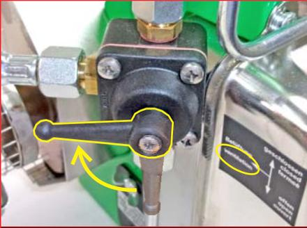
To stop fog, turn the Solution Tap Valve handle to VENTILATION. Wait until fog stops completely.
