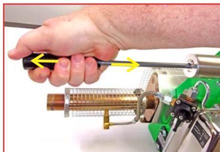
While pressing the Starter Button, cycle Air Pump until the fogger starts. Keep pumping for 10 sec. after it starts.
