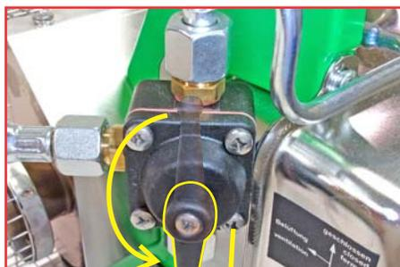
**To start fogging, turn the valve handle straight down to OPEN**
