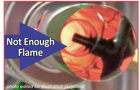
**If the flame does not reach the end of the Resonator you must increase the amount of fuel with the Regulating Needle.**
