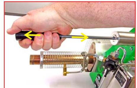
With the Fuel Button OFF, hold the Starter Button ON and pump the Air Pump until the fogger stops popping.
