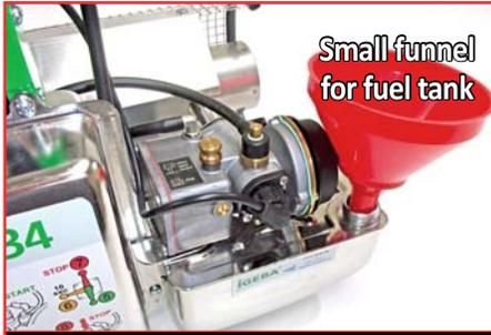
Gasoline goes in the small tank at the rear of the fogger. Use the small funnel to fill the tank and reduce spills.
