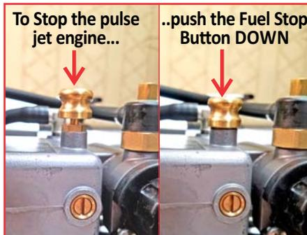
To stop the fogger, push the Fuel Stop Button DOWN which stops the gas to the engine.
