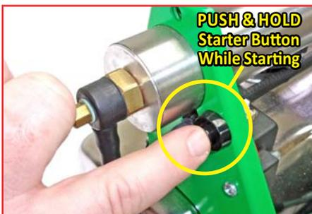
**PUSH and HOLD** the Starter Button while cycling the Air Pump. Hold Starter Button for 10 seconds after fogger starts.
