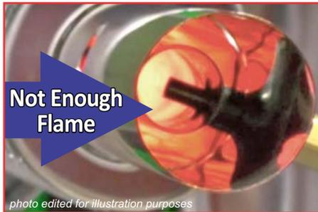
**If the flame does not reach the end of the Resonator you must increase the amount of fuel with the Regulating Needle.**
