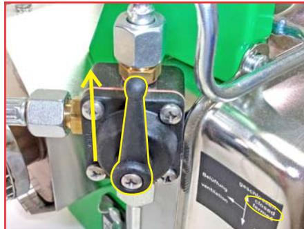
Before starting, make sure the Solution Tap Valve is CLOSED (handle points up).
