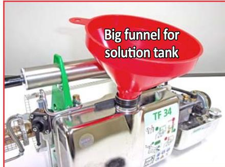
The fogging chemical goes in the larger tank. Use the big funnel to fill the tank.
