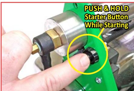
**PUSH & HOLD** the Starter Button while cycling the Air Pump. Hold Starter Button for 10 seconds after fogger starts.
