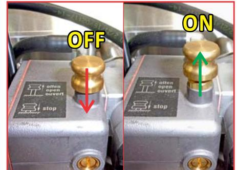
To start the fogger, you need fuel. Pull the Fuel Stop Button UP which allows fuel to flow.
