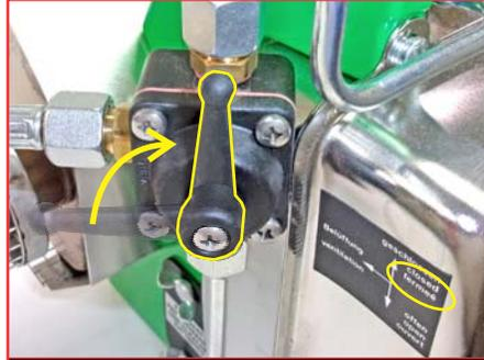
After VENTILATION, turn the Solution Tap Valve handle up to the CLOSED position.
