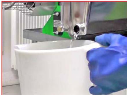
Before storing your fogger, be sure to drain and flush both Solution and Fuel tanks.
